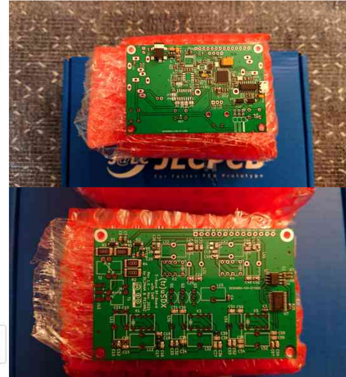
(tr)uSDX partly populated PCBs Produced and delivered by JLCPCB.
